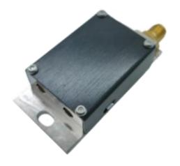
According to the existing material characteristics, Goptica designed AOTF products based on TeO2 shear wave acoustic mode. The wavelength range covers 350-2500 nm. Optimum performance is achieved in each wavelength range and meets most applications: resolution as low as 1 nm, FOV Angle up to 20 degrees, and aperture up to 10 mm.
